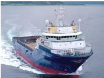
Stril Pioner DF-electric offshore supply vessel Simon Møkster Kleven Verft 4x 6R32DF 4x 16'500 running hours
