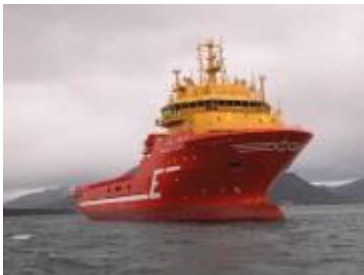
Viking Energy DF-electric offshore supply vessel Eidesvik Kleven Verft 4x 6R32DF 4x 19'500 running hours
