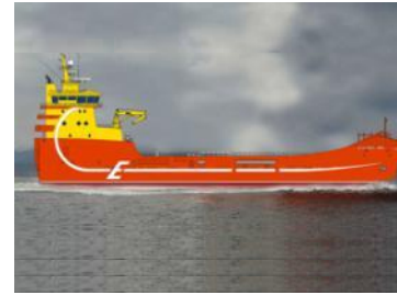
Viking tbn (Gass Avant) hull 29 DF-electric offshore supply vessel Eidesvik West Contractors 4x 6R32DF Ship delivery 2007
