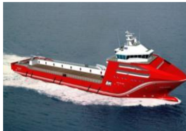
DF-electric offshore supply vessel Aker yards 3x W6L34DF Engines delivery 2010
