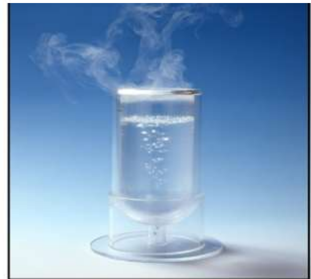
Figure 1. LNG "boiling" at atmospheric pressure and temperature (Source: Osaka Gas Co. Ltd.)
