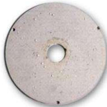
SIGMAGLIDE® Disk After rotating at 17 knots
