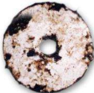
SIGMAGLIDE® Disk 2 years' exposure
